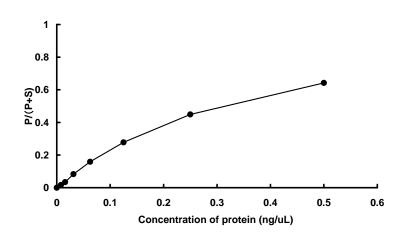
The activity was measured by off-chip mobility shift assay. The enzyme was incubated with fluorecence-labeled substrate and Mg(or Mn)/ATP. The phosphorylated and unphosphorylated substrates were separated and detected by LabChip<sup>™</sup>3000.
