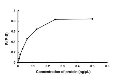
The activity was measured by off-chip mobility shift assay(MSA). The enzyme was incubated with fluorecence-labeled substrate and Mg(or Mn)/ATP. The phosphorylated and unphosphorylated substrates were separated and detected by MSA device.
