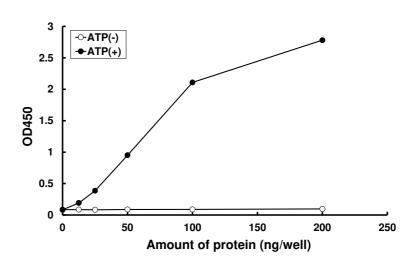
The activity was determined by ELISA. The enzyme was incubated with biotinylated substrate protein/peptide, and after stopping kinase reaction by EDTA, the reaction solution was transferred into streptavidin-coated plate. Phosphorylation was detected by antiphospho antibody and HRP-labeled anti-rabbit IgG(or HRP-labeled anti-mouse IgG).
