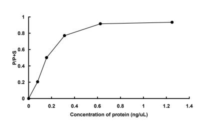
The activity was measured by off-chip mobility shift assay. The enzyme was incubated with fluorecence-labeled substrate and Mg(or Mn)/ATP. The phosphorylated and unphosphorylated substrates were separated and detected by LabChip $^{\text{TM}}$ 3000.
