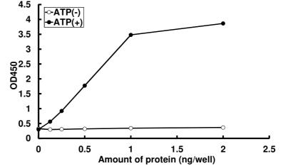
Purity: 69 % The purity was assessed by SDS-PAGE/CBB staining. The activity was determined by ELISA. The enzyme was incubated with biotinylated substrate protein/peptide, and after stopping kinase reaction by EDTA, the reaction solution was transferred into streptavidin-coated plate. Phosphorylation was detected by anti-phospho antibody and HRP-labeled anti-rabbit IgG(or HRP-labeled anti-mouse IgG).
