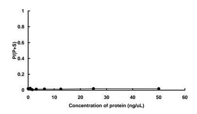
The activity was measured by off-chip mobility shift assay. The enzyme was incubated with fluorecence-labeled substrate and Mg(or Mn)/ATP. The phosphorylated and unphosphorylated substrates were separated and detected by LabChip $^{\text{TM}}$ 3000.
