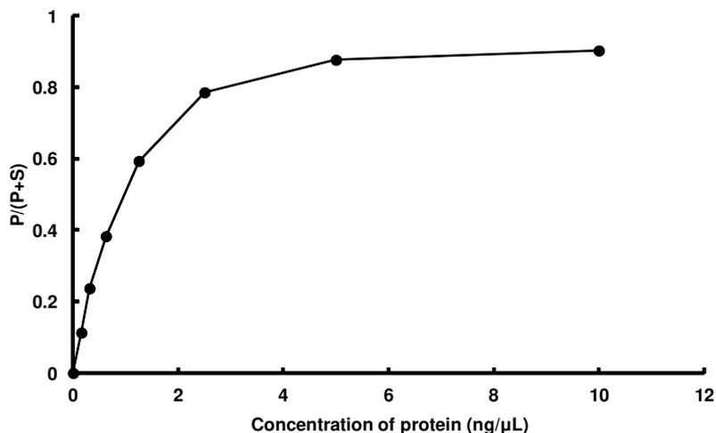
The activity was measured by off-chip mobility shift assay(MSA). The enzyme was incubated with fluorescence-labeled substrate and Mg(or Mn)/ATP. The phosphorylated and unphosphorylated substrates were separated and detected by MSA device.
