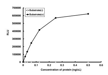
The activity was determined by ADP-Glo™ Assay. The enzyme was incubated with Lipid substrate and Mg(or Mn)/ATP. The phosphorylation was detected by the ADP-Glo™ Kinase Assay technology (luminescent ADP detection assay).
