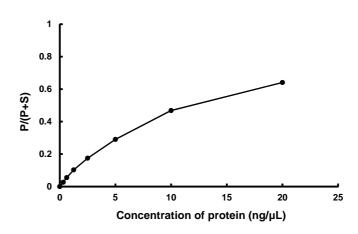
The activity was measured by off-chip mobility shift assay(MSA). The enzyme was incubated with fluorecence-labeled substrate and Mg(or Mn)/ATP. The phosphorylated and unphosphorylated substrates were separated and detected by MSA device.
